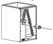
Fig. 6 - Liquid Line Filter Drier
